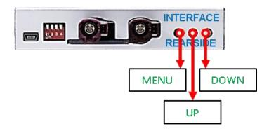
The picture settings are adjustable by the 3 push-buttons at the rear-side of the video-interface. Press the MENU button to open the OSD settings menu or to switch to the next menu item. Press UP and DOWN to change the selected value. The buttons are placed inside in the housing to avoid accidental changes during or after the installation. Picture settings must be done separately for AV1 and AV2 while the corresponding input is selected and visible on the monitor.
