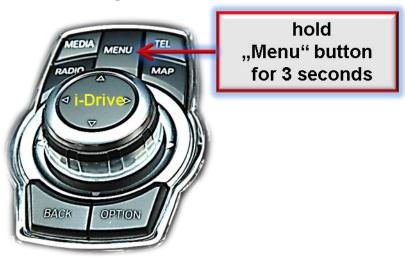
To switch the interface's activated video sources; the factory infotainment buttons can be used.
