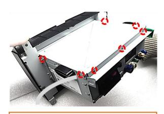
Lead the 20pin picture signal cable out of the housing at the indicated point, without jamming it and fix the housing cover by the 7 screws.
