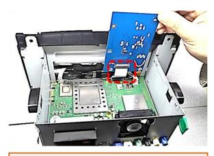
Connect the opposite side of the enclosed 40pin ribbon cable to the ribbon cable base "PCB-IN" of the daughter PCB's bottom side.
