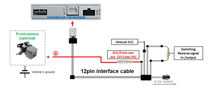
1 The red power supply output ACC/front cam out 12V (max 3A) can be used to power a front camera. If Dip 1 is set to ON (black 8 dips), the power supply output gives +12V (max 3A) when reverse gear is engaged plus 10 seconds delay after reverse gear is disengaged.
