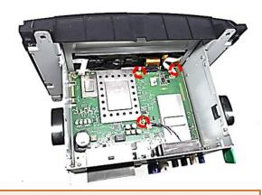
Unscrew the 3 screws at the indicated points and replace them with the enclosed spacers.
