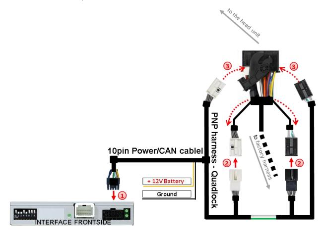
1 Connect the female 10pin connector of the 10pin Power / CAN cable to the 10pin connector of the video interface.
