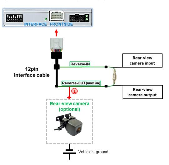
Additionally, the +12V (max. 3A) power supply for the rear-view camera can be taken from the green wire of the 12pin interface cable.
