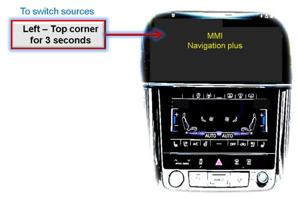
A long press in the touch display's left upper edge switches the interface's activated video sources.
