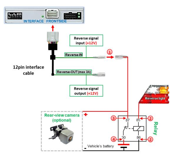
Disconnect the green cable's preconnected male- and female connectors of the 12pin interface cable and connect the green input cable "Reverse-IN" to the output connector (87) of the relay.
