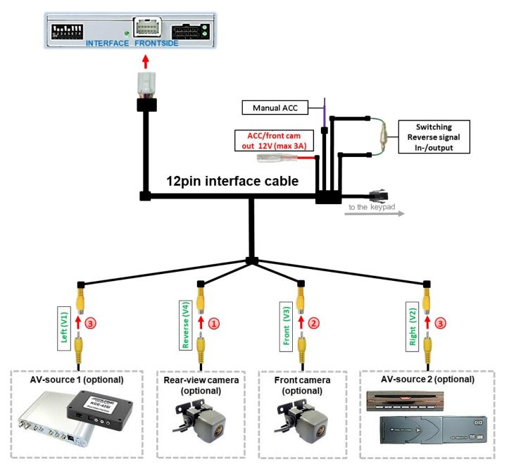
Connect the video RCA of the Rear-view camera to the 12pin interface cable's female RCA connector **"Reverse V4**.
