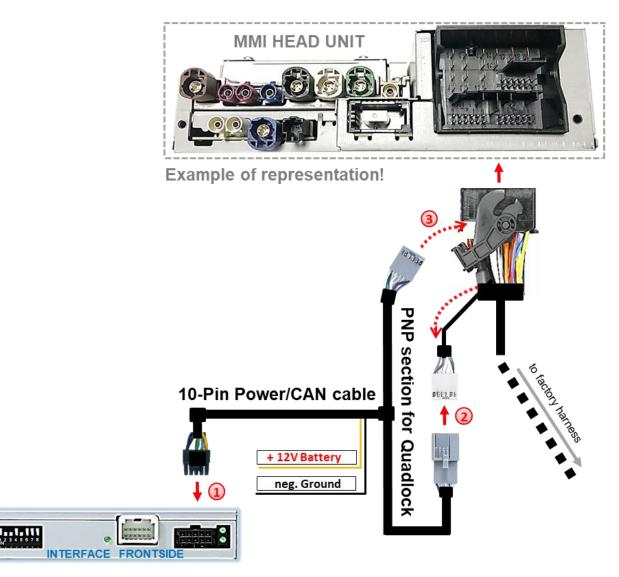
Connect the 10pin power/CAN cable's female 10pin connector to the 10pin connector of the video interface.
