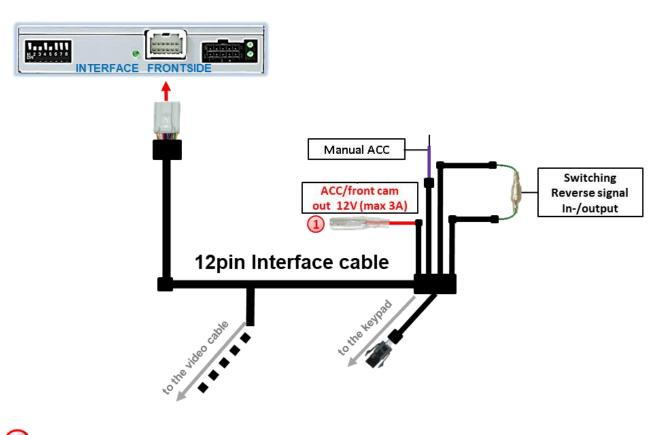
The red power supply output ACC/front cam out 12V (max 3A) can be used to power an external source and has a different assignment depending on the position of dip switch 1 (of the black 8 dips):
