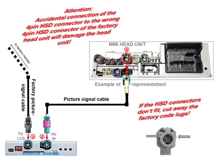
Disconnect the factory picture signal cable's **black** female HSD connector at the rear-side of the head unit and connect it to the waterblue coloured male HSD connector **"TO LCD"** of the video interface.
