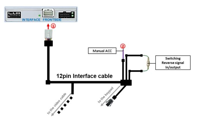
If, after connecting the PNP harness, no interface LED lightens up while the ignition is turned on, the purple coloured wire Manual ACC of the 12pin interface cable has to be connected additionately to ACC or S-contact terminal 86s +12V (e.g. glove compartment illumination). 2.5. Power supply output
