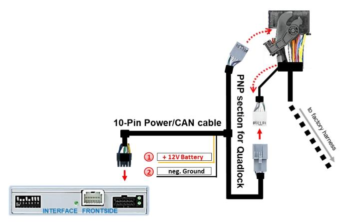
Connect the single yellow wire of the 10pin power/CAN cable to +12V permanent and stabile power supply.
