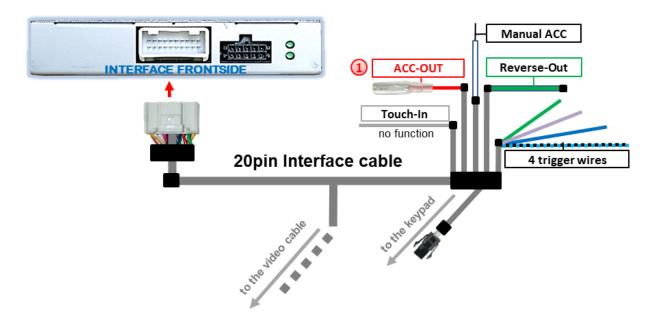
1 The red power supply output "ACC-out" can be used to power an external source.
