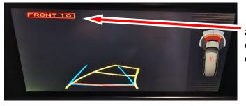
and additionally 10, 15 or 20 seconds delay after reverse gear is disengaged for the front camera.
