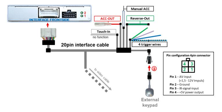
Connect the keypad's female 4pin connector to the 20pin interface cable's male 4pin connector.
