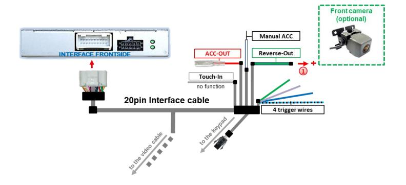
The green power supply output "Reverse-Out" can be used to power a front camera. If Dip 1 is set to ON (of the black 8 dips), the power supply output supplies +12V (max 3A) when the reverse gear is engaged ...
