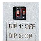
After each Dip-switch-change a power-reset of the Can-box has to be performed!
