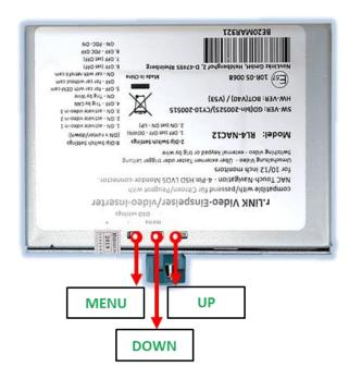
The picture settings can be adjusted by the 3 buttons on the video-interface. Press the MENU button to open the OSD settings menu. To switch to the next menu item, pressing UP and DOWN will change the selected value. The buttons are embedded in the housing to avoid accidental changes during or after installation. The picture settings have to be done separately for AV1 and AV2 while the corresponding input is selected and visible on the monitor.
