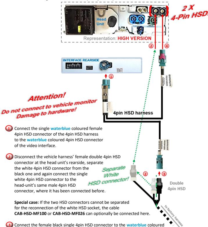
Connect the opposite waterblue coloured female 4pin HSD connector of the 4pin HSD
