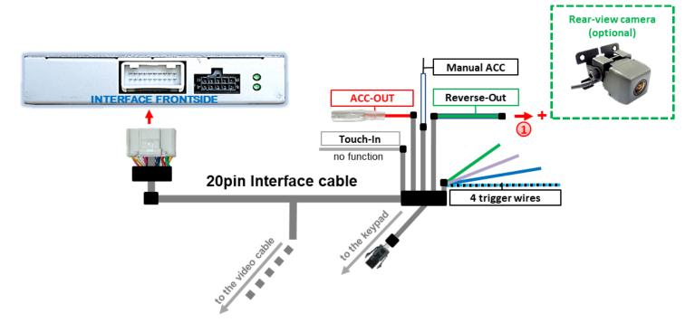
The 12 V power supply for the rear-view camera (max 3A) has to be taken from the green wire "Reverse-OUT" of the 20pin cable to avoid an unnecessary, permanent power supply to the camera electronic.
