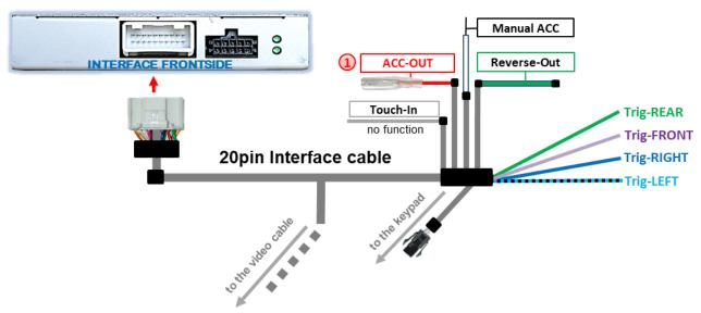
1 Power is supplied to the mirror cameras via the red cable "ACC-out".
