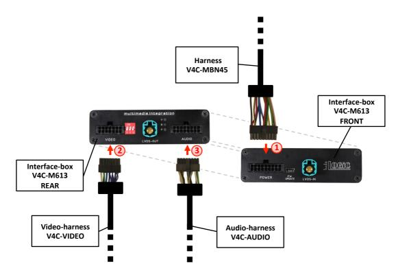
Connect female 18pin Micro-Fit connector of harness V4C-MBN45 to the male 18pin Micro-Fit connector (POWER) on the front of the interface-box V4C-M613.
