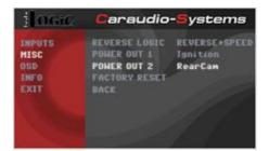
On some vehicles the reverse light signal doesn't exist on the CAN-bus. Connect the white wire of harness V4C-MBN45 to reverse light signal (+12V of reverse light) if the v.LOGiC doesn't switch to the rear-view camera automatically after the described OSD-setup (see next chapter).
