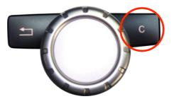
In the vehicle's **Audio menu**, activate **AUX** and after it **long press C button** to choose the v.LOGiC as current AV-source.
