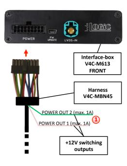
1 You can configure the both +12V trigger outputs separately. The pink wire is POWER OUT 1 and the green wire is POWER OUT 2.
