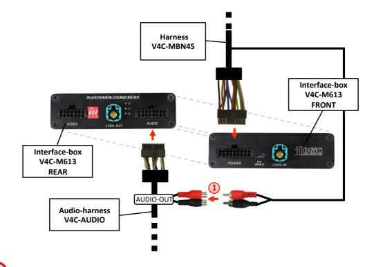
Connect the audio-RCA of harness V4C-MBN45 to the female RCA-connectors AUDIO OUT of the audio-harness V4C-AUDIO.
