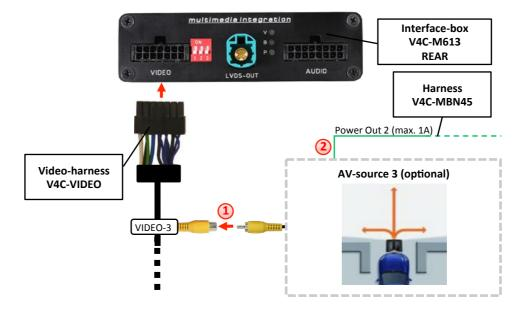
Connect the video RCA of the after-market front camera to the female RCA connector VIDEO-3 of the video-harness V4C-VIDEO.
