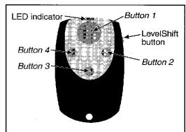
To transmit channel 9, 10, 11 or 12: Press the LevelShift button twice. This shifts buttons 1–4 to level 3 (channels 9–12). Then press the corresponding button within the next 7 seconds. For instance, to transmit channel 10, press the LevelShift button twice, then press button 2. While you transmit, you'll notice that the LED blinks three times, pauses, blinks three times, etc.: this indicates level 3.
