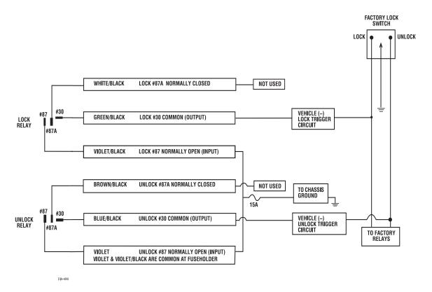
Wiring Diagram C, Directly-Wired Reversing-Polarity Switch Circuits
