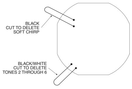
The 514LN Soft-Chirp siren will chirp 6dB softer than its full-volume output. This means that arming and disarming chirps, Warn-Away chirps, and the first stage of the two-stage progressive door trigger will be 6dB quieter than the siren's constant output.
