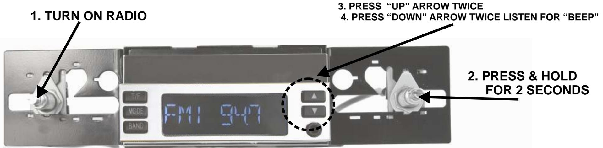
1. TURN ON RADIO BY PRESSING LEFT CENTER SHAFT BUTTON
