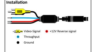
**Note:** If the camera is powered by reverse gear lamp signal, we recommend to install a relay between the power supply of the reverse signal and the power supply of the camera, to ensure a stable and uninterrupted power supply and to avoid unwanted errors in the vehicle computer.
