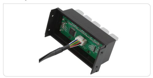
If the Radio Face is still connected to the Radio Body, remove the two screws on each side of the face and gently detach the Radio Face from the Radio Body. Remove the white connector from the PC board of the Radio Face. Plug the large white connector of the extension cable into the Radio Face.
