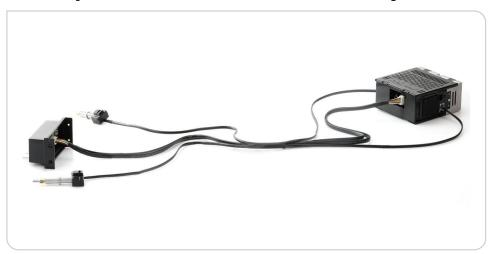
Plug the RJ-11 telephone plug connectors into the sides of the Radio Body. Then plug the large white connector into the Radio Body.
