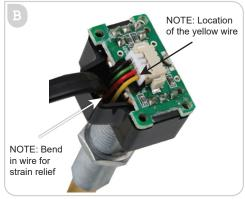
Unplug the white connector from the PC board in the rear of the shaft. Notice the bend in the wire; you will need to bend the wiring of the new extension cable when installing it. (NOTE: the bend in the wire acts as a strain relief for the cable when the back is re-installed).
