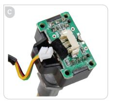
Plug the extension cable's connector into the PC board of the shaft. Please do not force the connector into the socket; it only installs oneway; see the location of the yellow wire in the image above.
