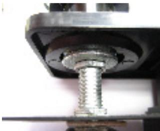
Nuts/Washers Installed Between
