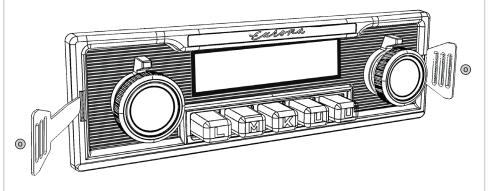
If adjustments are needed, use the included DIN Keys to remove the assembly from the DIN Sleeve.
