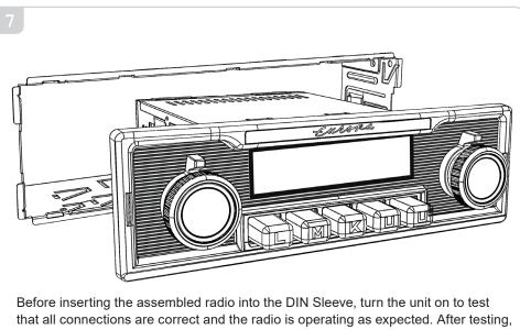
slide the radio assembly into the DIN Sleeve until the unit clicks into place.
